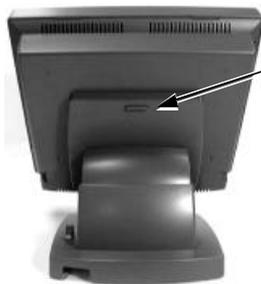
Press the Lock/Release button and lift the main unit to detach it from the stand assembly.
