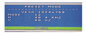
**RECALL** Returns the adjustments back to factory settings if the monitor is not operating at its original factory settings. Select RECALL using the [+] or [–] button, then press [Menu] button to reset the settings.
