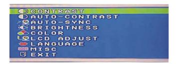
**CONTRAST** Adjusts the contrast level of the screen image. Under Main Menu, select CONTRAST using the [+] or [-] button, then press [Menu] button to activate the function. Press the [+] button to increase contrast, [-] button to decrease contrast shown below. Press [Menu] to return to Main Menu.
