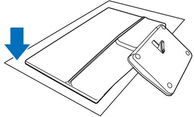
2. Hold the monitor and base with both hands. Gently bend the base vertically down to a fixed angle.
