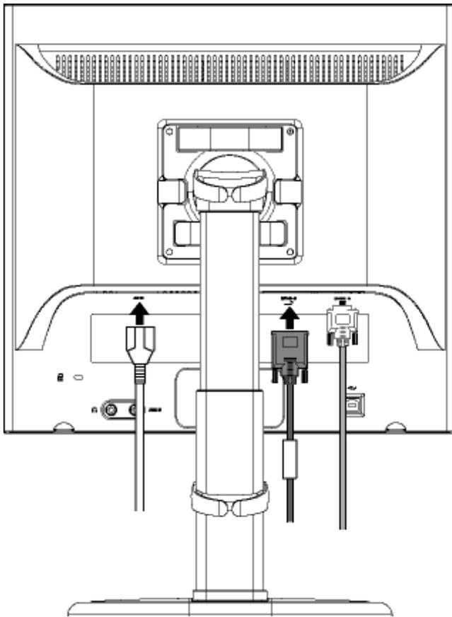
1) Plug in the cables into connectors.
