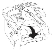
3 Remove the toner cartridge by gripping the handle in the middle and pulling it forwards out of the device
