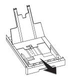
3 Adjust the length of the paper tray to the printer paper. Press the lock key on the base of the paper tray. Slide the rear panel until it snaps into the suitable marking: Legal = LG, A4 = A4, A5 = A5, Letter = LE, B5 = B5.
