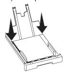
**6** Push the paper tray into the device all the way to the stopping point.
