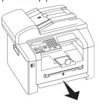
**3** Push the paper tray into the device all the way to the stopping point.
