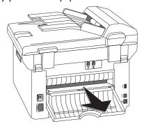
4 Close the paper jam flap. The fuser levers will automatically fold into starting position when the paper jam cover is closed.
