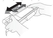
**6 Only after** completely pull off the protection strip located on the left side of the cartridge.
