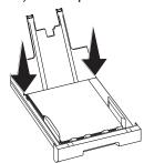
**8** Push the paper tray into the device all the way to the stopping point.
