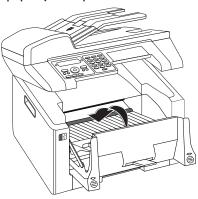
7 Place the toner cartridge into your device. The cartridge should snap securely into position.
