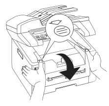
3 Remove the toner cartridge by gripping the handle in the middle and pulling it forwards out of the device
