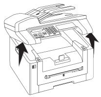
2 Open the device by lifting the device cover forwards
