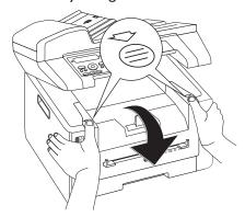
3 Remove the toner cartridge by gripping the handle in the middle and pulling it forwards out of the device
