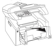
4 Remove the tape and protective paper, but do not remove the protective strip from the cartridge yet.
