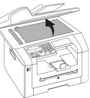
2 Lay the document onto the scanner glass with the written side down.
