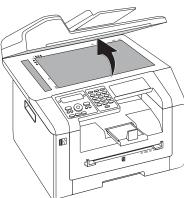
2 Carefully wipe the scanner glass of the flatbed scanner (1) and the automatic document feeder (2) with a lint-free cloth.
