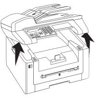
2 Open the device by lifting the device cover forwards
