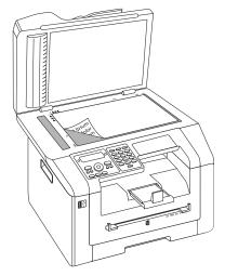
3 Align the document with the rear left corner of the scanner glass (arrow marks). The markings on the scanner border for the A4 and A5 formats will help you to position the document correctly.
