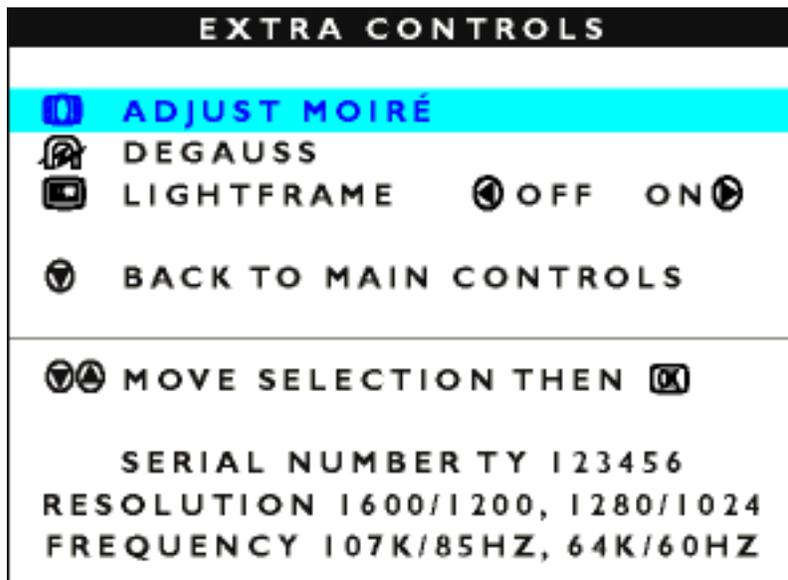
4) Press the
