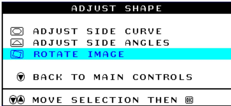
5) Press the
