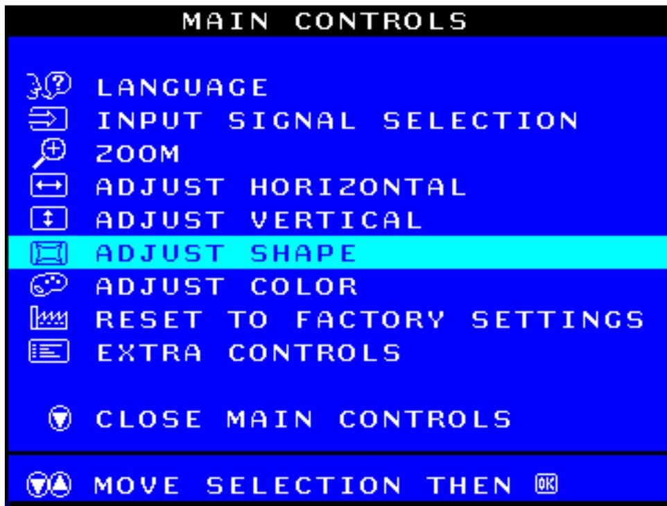
3) Press the
