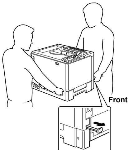
Even if an optional lower feeder unit is installed, be sure to lift the printer as shown below. Do not grasp the grip of Tray 2, 3 or the right side cover; otherwise, the lower feeder unit may be damaged.
