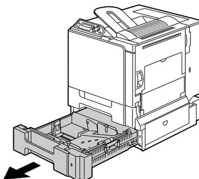
**2** Press down on the media pressure plate to lock it into place.
