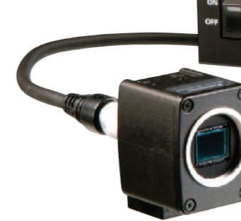
1/2-type 3CCD Color Camera Head GP-US522HB
