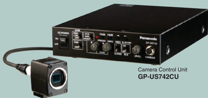
1/2-type 3CCD Color Camera Head GP-US522HB
