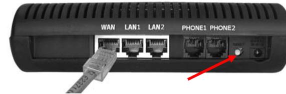
Hold this button down for about 7-10 seconds until you see all the LED lights turn off except for the POWER light. (This is necessary in order to clear the cache memory upon upgrading. After the device reboots, you will need to re-enter your device configuration.)
