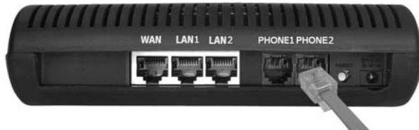
3. Connect one end of an Ethernet network cable to the LAN port of the ATA. Connect the other end to the Ethernet port of your PC.
