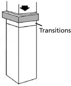
Counterflow Furnace- Mounted horizontally in return duct- just above the furnace.
