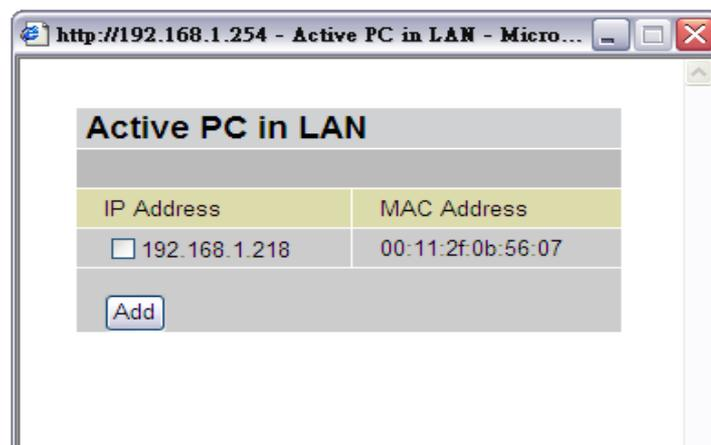
Active PC in LAN displays a list of individual Ethernet device's IP Address & MAC Address which connecting to the router.
