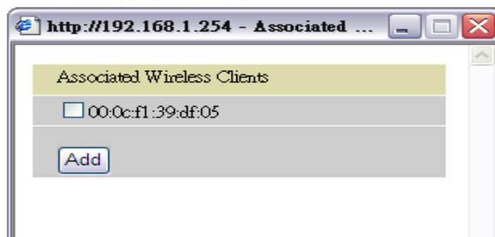
Associate Wireless Client displays a list of individual wireless device's MAC Address that currently connects to the router.
