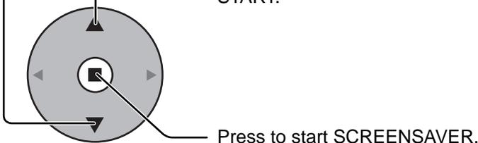
The menu screen will disappear and the SCREENSAVER will be activated. **To stop the SCREENSAVER under ON, press the R button.**
