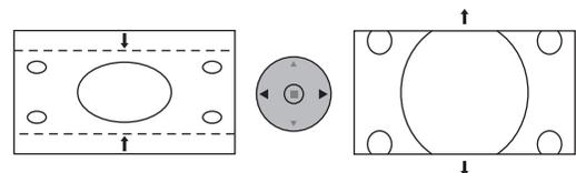
**CLOCK PHASE** (RGB/PC in mode) Eliminate the flickering and distortion.
