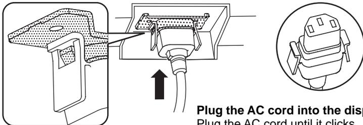
**Plug the AC cord into the display unit.**
