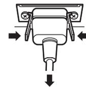
Unplug the AC cord pressing the two knobs.
