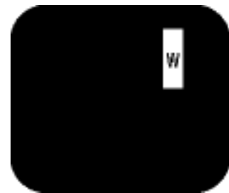
Three adjacent lit subpixels (one white pixel)
