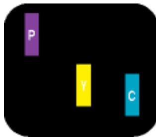
Two adjacent lit subpixels: - Red + Blue = Purple - Red + Green = Yellow - Green + Blue = Cyan (Light Blue)
