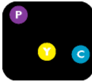
Two adjacent lit subpixels: - Red + Blue = Purple - Red + Green = Yellow - Green + Blue = Cyan (Light Blue)
