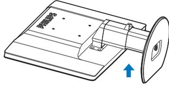
3. Release the lock of base stand then pull the base stand away from the base column.
