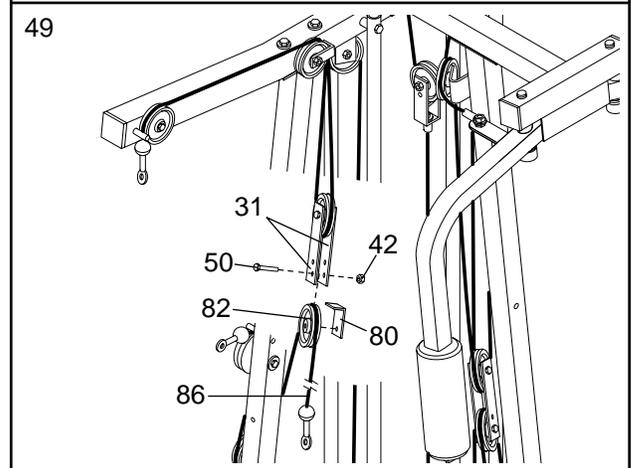
50. Wrap the Low Cable (86) around a 3 1/2" Pulley (82). Attach the Pulley to the Ab Upright (1) with the 3/8" x 3 1/2" Bolt (66), a 3/8" Washer (38), and a 3/8" Nylon Locknut (42). **The ball on the Cable must be on the indicated side of the Pulley. Be sure that the Cable and Pulley move smoothly and that the Cable is between the Pulley and the post.**
