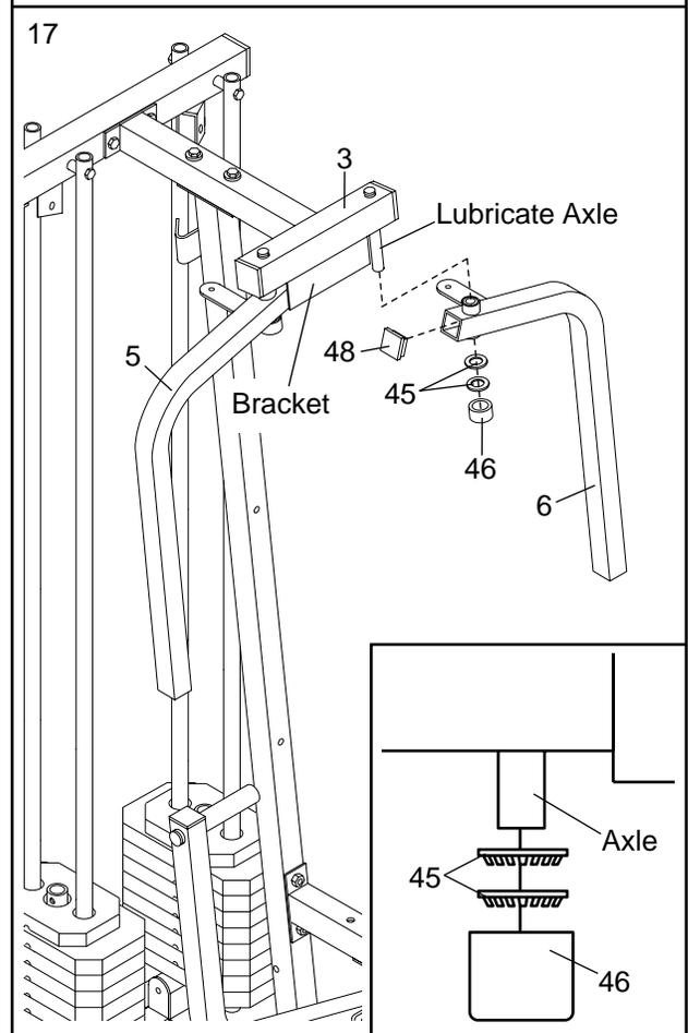
**IMPORTANT NOTE: Before assembling the 1" Retainers (45) used in this step, be sure that you thoroughly understand the step. The Retainers can be assembled only once. If they must be removed, you will need to order new Retainers.**
