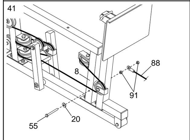
42. **Locate the High Cable (85)—this is the shortest remaining cable.** Wrap the High Cable around a 3 1/2" Pulley (82). Attach the Pulley to the Top Frame (2) with a 3/8" x 3 1/2" Bolt (66), a 3/8" Washer (38), and a 3/8" Nylon Locknut (42). **Be sure that the end of the Cable with the ball is on the indicated side of the Pulley and that the Cable is between the Pulley and the post.**
