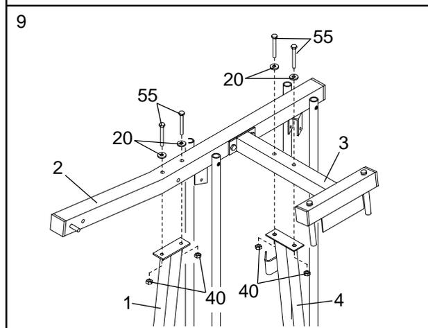
Attach the Butterfly Frame (3) to the Leg Press Upright (4) with two 5/16" x 2 3/4" Bolts (55), two 5/16" Washers (20), and two 5/16" Nylon Locknuts (40). **Do not tighten the Nylon Locknuts yet.**
