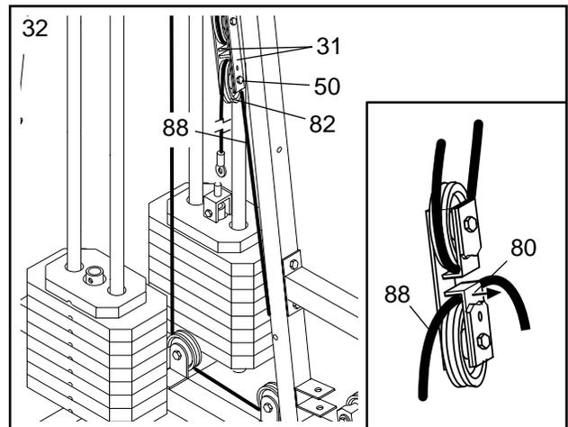
33. Route the Press Cable (88) around a 3 1/2" Pulley (82). Attach the Pulley and a Cable Trap (80) to the Leg Press Upright (4) with a 3/8" x 3 1/2" Bolt (66), a 3/8" Washer (38) and a 3/8" Nylon Jam Nut (43). **Be sure that the Cable Trap is turned to hold the Cable in place.**
