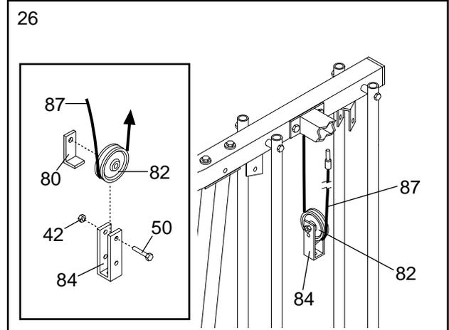
Route the Rear Cable (87) through the Large "U" Bracket (84) and the 3 1/2" Pulley (82). **Be sure that the Cable is in the groove of the Pulley and that the Cable and Pulley move smoothly.**
