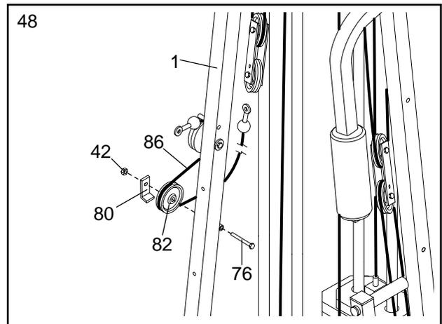
49. Remove the indicated 3/8" x 2" Bolt (50), the 3/8" Nylon Locknut (42), the 3 1/2" Pulley (82), and the Cable Trap (80) from the indicated Pulley Plates (31). Lay the Low Cable (86) over the Pulley. Reattach the Pulley and the Cable Trap to the lowest hole in the Pulley Plates with the Bolt and the Nylon Locknut. **Make sure that the Cable Trap is turned to hold the Cable in place.**
