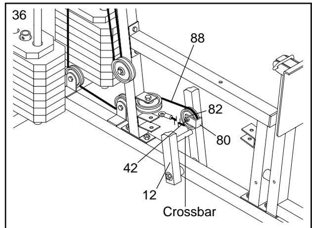
37. Wrap the Press Cable (88) around a "V" Pulley (81). Attach the "V" Pulley to the lower bracket on the Leg Press Upright (4) with a 3/8" x 2" Bolt (50) and a 3/8" Nylon Jam Nut (43).
