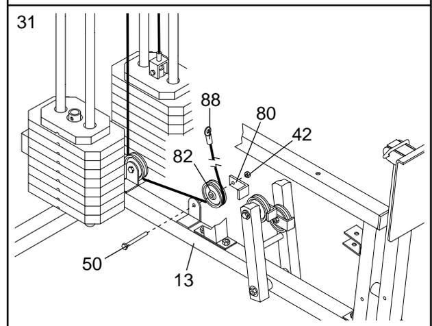
32. Route the Press Cable (88) over the indicated 3 1/2" Pulley (82) attached to the Pulley Plates (31). **The Cable must be routed from the direction shown.** Refer to the inset drawing. **Be sure that the Cable is between the Cable Trap (80) and the Pulley, and that the Cable Trap is positioned to hold the Cable in place.**
