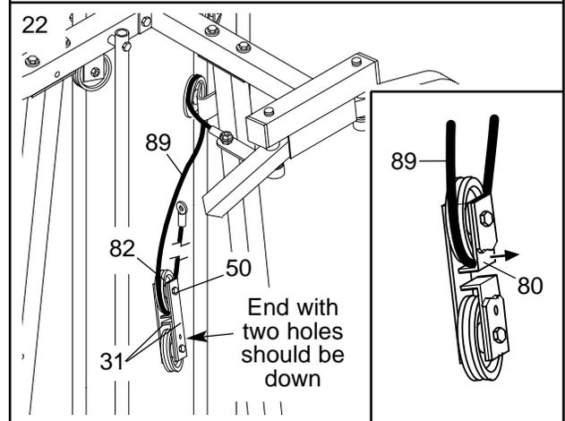
Tighten the 3/8" x 2" Bolt (50) and the 3/8" Nylon Locknut (not shown).
