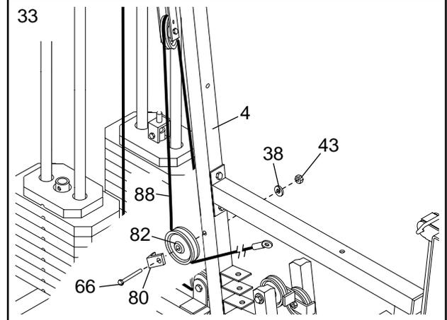
34. Route the Press Cable (88) over the indicated 3 1/2" Pulley (82) attached to the Press Frame (12). Tighten the 3/8" x 3 1/2" Bolt (66) and the 3/8" Nylon Locknut (not shown).
