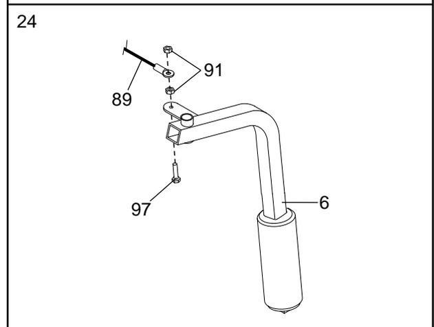
Slide the free end of the Butterfly Cable (89) onto the 5/16" x 1" Bolt (97). Thread another 5/16" Nylon Jam Nut (91) onto the Bolt, **but do not fully tighten it. Leave enough room between the two Jam Nuts for the Cable to pivot.**
