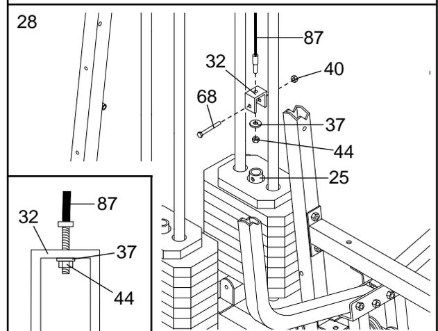
Attach the Small "U" Bracket (32) to the indicated Weight Tube (25) with a 5/16" x 1 3/4" Bolt (68) and a 5/16" Nylon Locknut (40).
