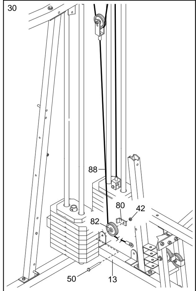
31. Wrap the Press Cable (88) around a 3 1/2” Pulley (82). Attach the Pulley and a Cable Trap (80) to the other bracket on the Press Base (13) with a 3/8” x 2” Bolt (50) and a 3/8” Nylon Locknut (42). **Be sure that the Cable Trap is turned to hold the Cable in place.**
