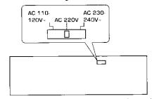
Move switch lever to match your line voltage with a small screwdriver or other pointed tool.
