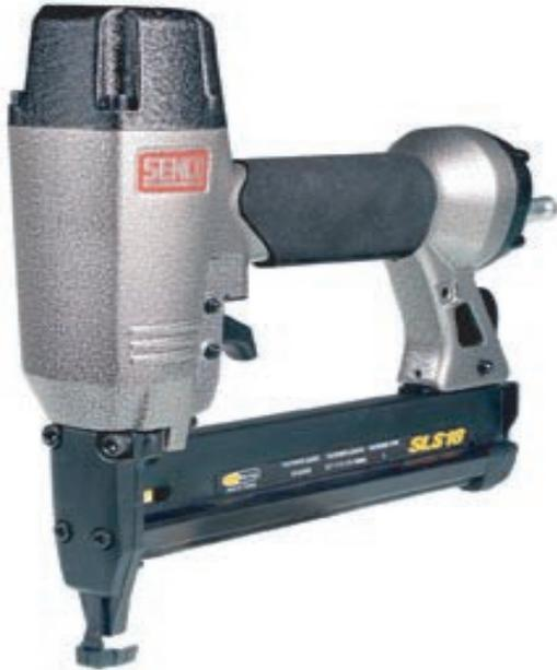
The versatile SLS18 finish stapler weighs just 2.9 lbs, but can drive 1/2" to 1-1/2" staples into hard woods. With either a dual or restrictive trigger, you can choose between high productivity or precision placement, making it the ideal stapler for a wide range of applications
