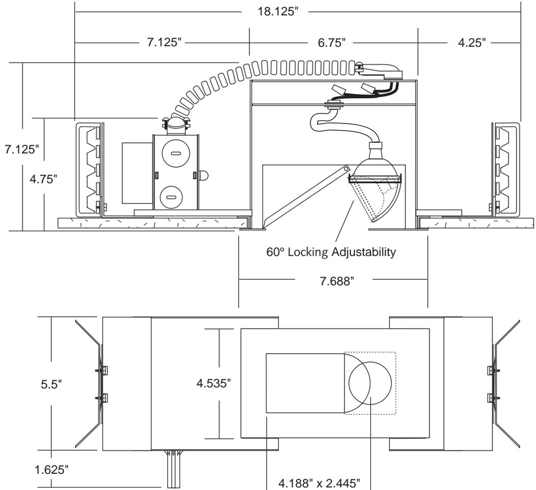
Provided with two (2) 14 gauge steel butterfly type brackets for black iron installations.
