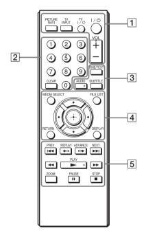
The VOL (volume) +, number 5, AUDIO, and buttons have a tactile dot. Use the tactile dot as a reference when operating the player.
