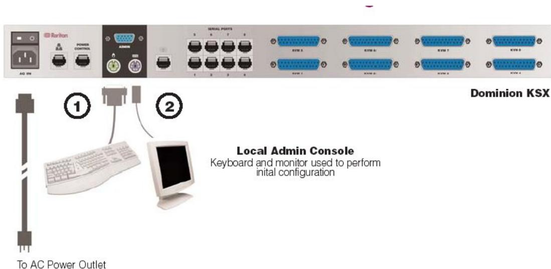
Figure 6 Dominion KSX Back panel Connections
