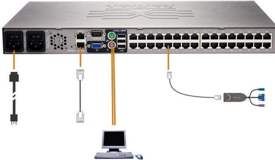
Figure 5 Dominion KX2 Connections
