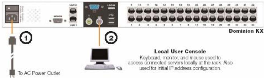
Figure 2 Dominion KX Physical Connections
