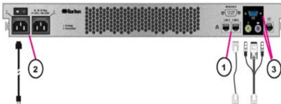
Figure 13 Physical Connections for CCSG G1 Units
