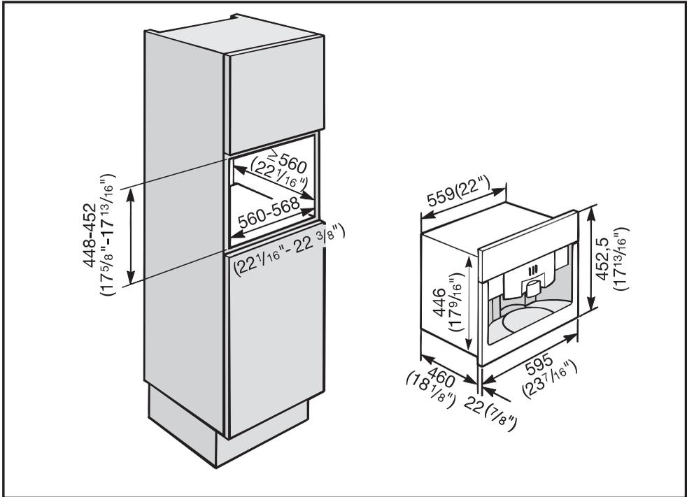
A combination with other Miele built in appliances is possible. If the machine is installed in combination with other appliances, it should be installed with a protective base between the appliance and the unit (exception: installation with a built-in plate warmer).
