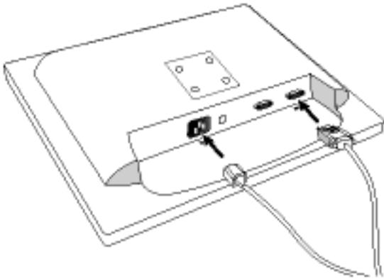
**1)** Put monitor face down on the safe surface and plug in the cables into connectors.
