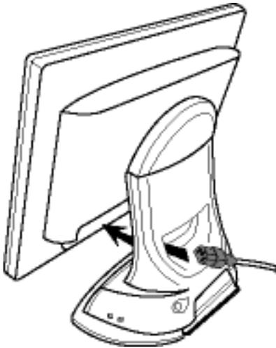
**5)** Thread power cable through the hole at the bottom of the base, and plug onto monitor firmly.
