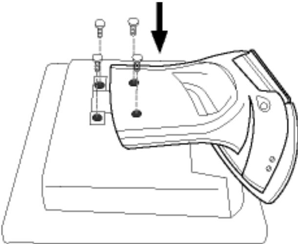
**2)** Mount the base onto the monitor body and fix four screws securely.
