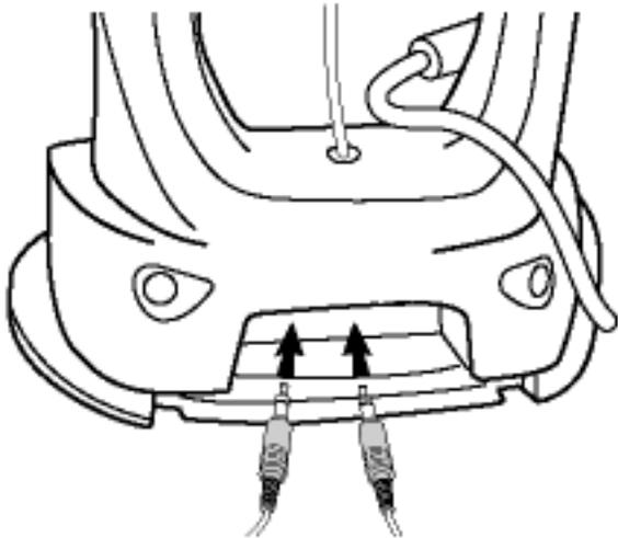
**6)** Connect microphone and audio cables onto the rear side of base if any.
