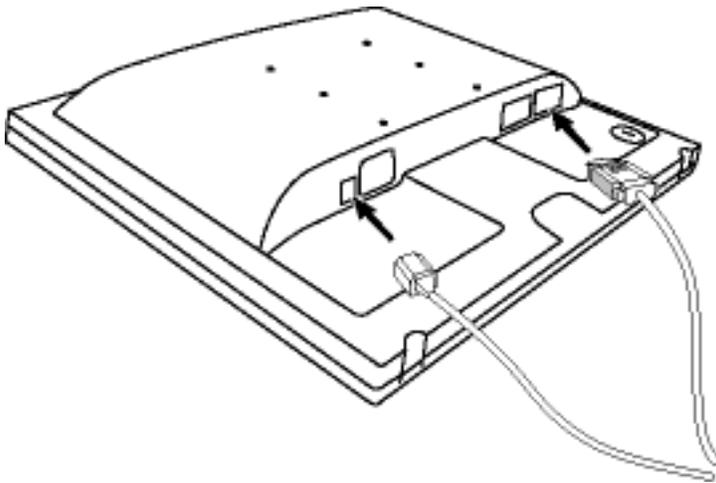
**1)** Put monitor face down on the safe surface and plug in the cables into connectors.
