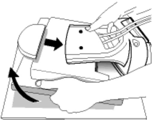
**3)** Lift the monitor body and thread all cables through the hole at the bottom of the base.
