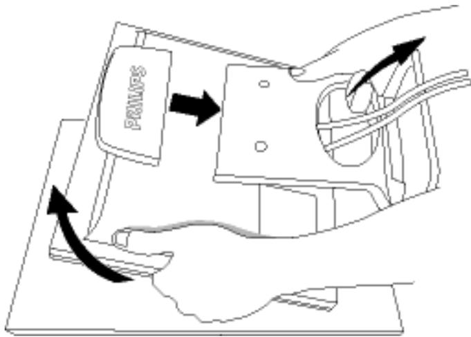
**3)** Lift the monitor body and thread all cables through the hole at the bottom of the base.
