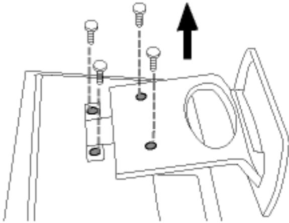
**3)** Unscrew the four screws of the base
