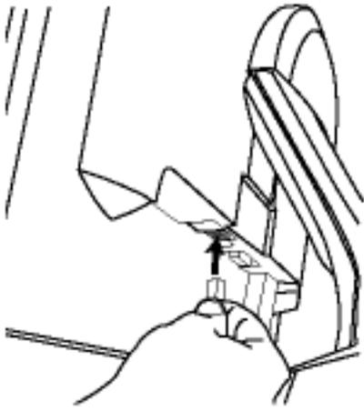
**4)** For Multimedia base, plug the flying DC power cable of base onto monitor.
