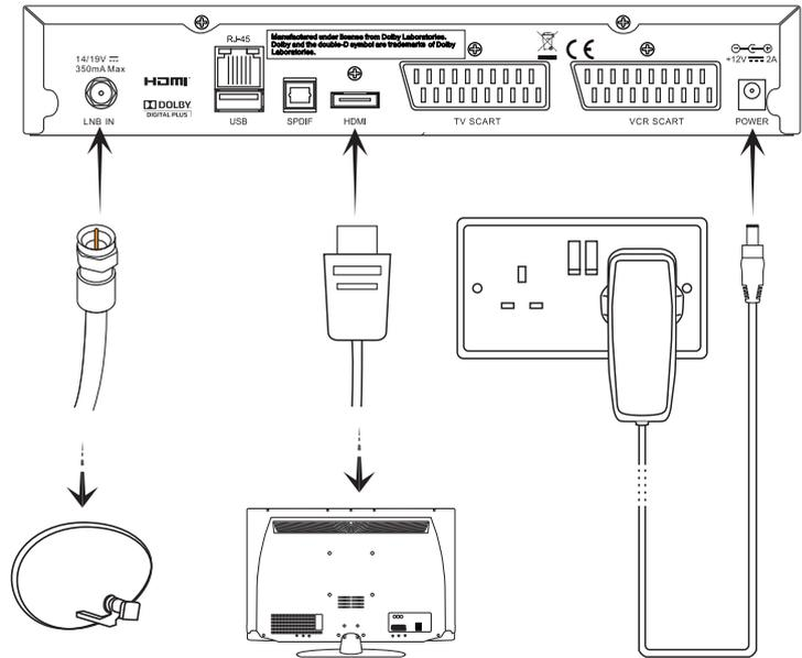
Connect the cable from your dish to the LNB IN socket at the back of the receiver (if the dish cable is fitted with a wall socket inside your home, you will need a connecting cable, which you can get from your installer).
