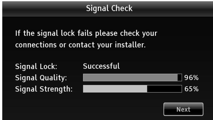
The signal check screen shows the strength and quality of the freesat signal received from your satellite dish. If the signal strength or quality is below 50%, you should check the satellite dish connection at the back of the receiver (switch the receiver off and reconnect the cable if necessary). If the connection is OK, consult your dealer or installer.
