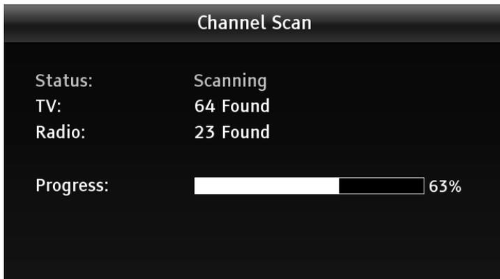
Your Plaza HD•S receiver will take a couple of minutes to find and store the available freesat channels. The number of freesat TV and radio channels found is shown on the screen as the scan proceeds, along with an indication of how far the scan has to go. When the scan is complete, press the **OK** button to proceed.
