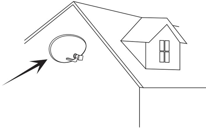
To receive freesat, you must connect your Plaza HD•S receiver to an appropriate satellite dish, fixed in position and accurately pointed at the 28.2° East satellite position.
