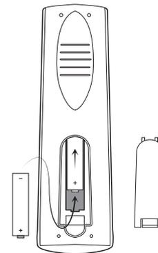
Take off the battery compartment cover from the back of the Plaza HD•S remote control by lifting it up while pushing the catch. Insert the two AAA batteries supplied, as shown on the inside of the compartment, and replace the compartment cover.
