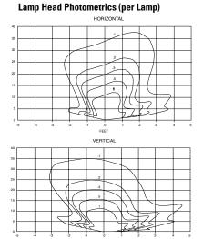
Complete Fixture consists of unit and two lamp heads. Lamp Head Photometrics (per lamp)
