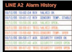
Alarm activation, check, and recovery can be recorded and displayed.
