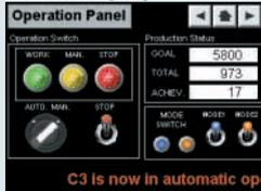
A flowing message of up to 64 characters (two-byte) can be displayed at the bottom of the screen. (128 messages)
