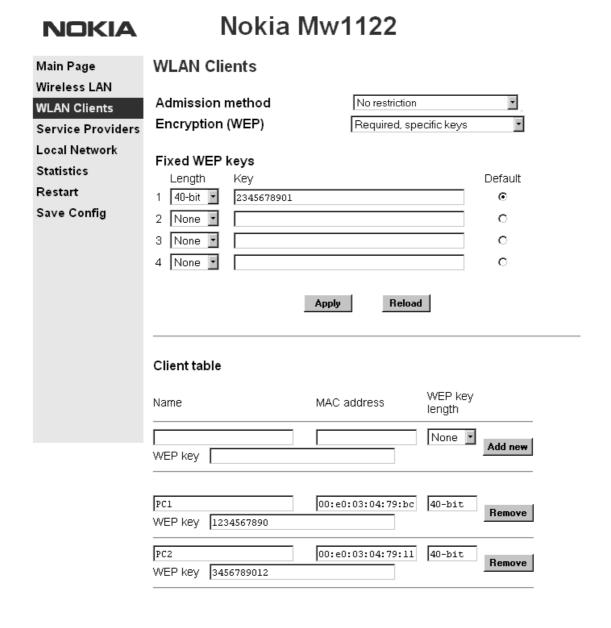
Figure 9 WLAN Clients page and station-specific key encryption
