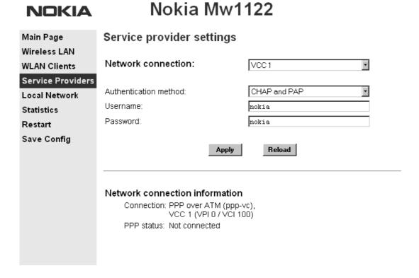
**Figure 10** Service Provider page with PPP configuration
