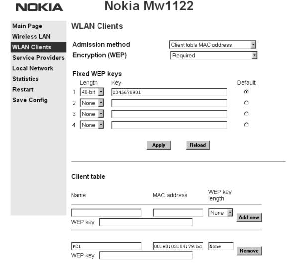
Figure 8 WLAN Clients page and default key encryption
