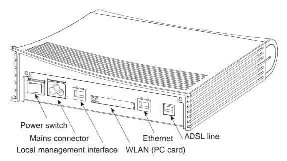
Figure 2 MW1122 back panel
