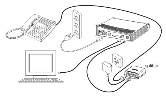
Figure 4 MW1122 and splitter connected
