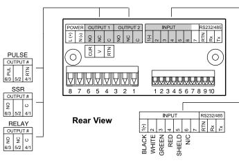
Refer to Operator's Manual for important Input Probe Note Shield wiring notes
