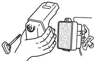
2. Use neutral detergent and warm water to clean the filter element. After cleaning, air dry the element completely and moisten with a small amount of motor oil.
