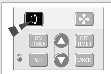
Depending on the position of the indoor unit on the wall of your room, you can adjust the position of the outer air flow blade on the bottom of the unit, thus increasing the efficiency of the air conditioner.
