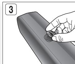
4. Use a coin turn the hole cover clock wise to fix it. (Turning it count-clock wise will loosen from the hole.)
