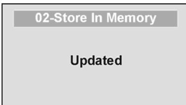
The value is stored in memory for later download to PC. If the memory is close to full the user will be warned and given the option to transfer all values to the PC or to clear the memory of all values.
