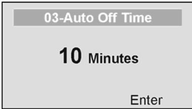
The user can determine how long the scale will operate before turning off automatically due to inactivity. Default time is 10 minutes. If the value is set to zero, the auto off function is disabled.
