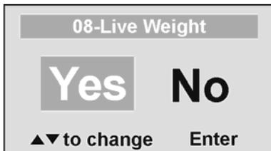
By selecting “Yes” the user can set the Live Weight mode to deactivate the motion-sensing mode. In the Live Weight mode the weight displayed will fluctuate with the patient’s movement; the scale will not lock on quickly to the weight as is the case in the motion-sensing mode. Press the REWEIGH button to operate the motion-sensing mode and to determine the correct weight on the screen. To revert back to motion-sensing mode, change the Live Weight setting to “No”.
