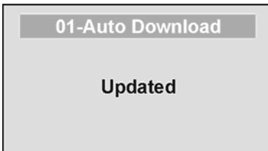
Automatic Download is the default option and will transfer the value to the PC as soon as the patient steps off the scale or when the user presses the HOLD/RELEASE button if it was kept in "HOLD". If no PC is connected, the value is not transferred and not stored and will be lost after the load is removed from the scale.
