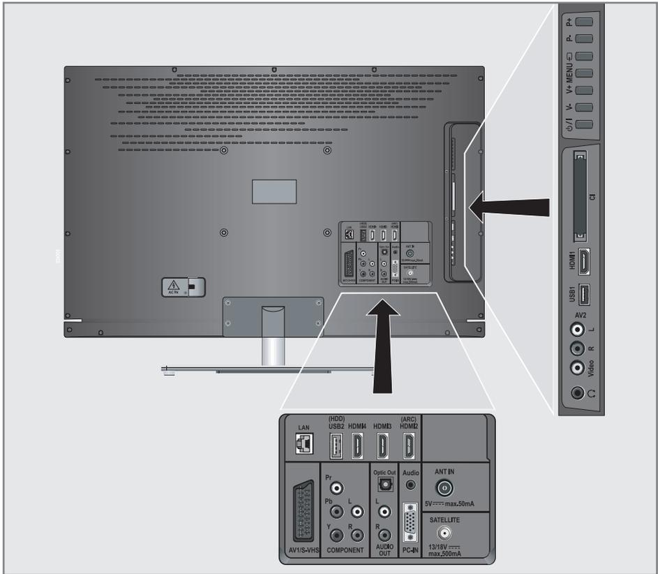
**AV1 / S-VHS** SCART socket (CVBS signal, RGB signal); Video and sound socket for S-Video camcorder.
