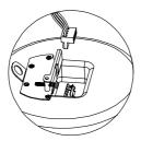
6. The terminal cover also acts as the strain relief. Rotate the cover clockwise and tighten the retaining screw.
