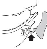
3. Turn the water chamber base upside down. Insert the latch's feet into the locking tabs. Push firmly and click into place.
