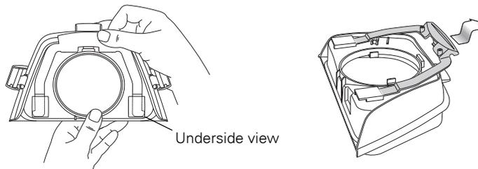
4. Disengage the catches from the sides of the water chamber base. Then, separate the inner and outer moulding of the catch, pull back the inner moulding and squeeze. The inner moulding will pop out.
