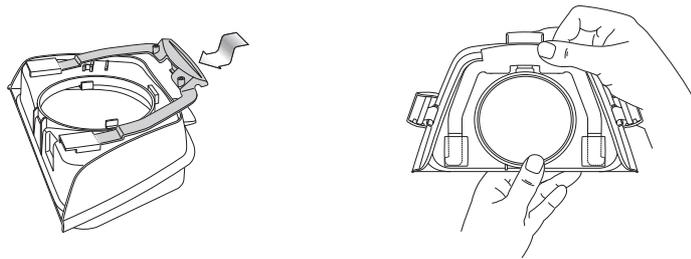
4. Refit the O-ring in the channel of the tub plate.
