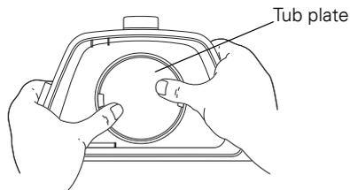
2. Remove the O-ring from the tub plate.
