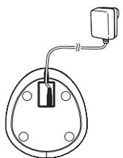
Connect the power adaptor to the cradle and a power outlet.
