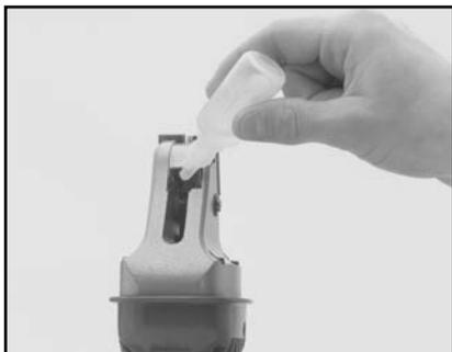
**Figure 5.** Lubricating shear.
