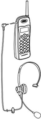
To connect the headset, open the rubber cover on the left side of the handset, then insert the headset's plug into the jack.
