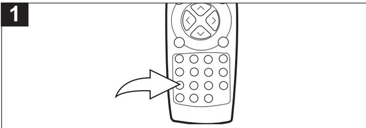
Press the PIP/POP button to turn picture-in-picture on; press a second time to turn picture on picture (split screen) on (this will show a picture next to a picture). Press a third time to turn PIP or POP off.
