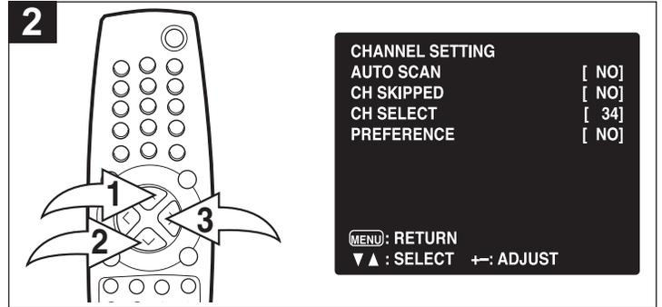
Press the CHANNEL UP ❶ or DOWN ❷ button until CHANNEL SETTING is selected, then press the VOLUME UP button ❸ to select it. Press the CHANNEL UP ❶ or DOWN ❷ button until CH SELECT is selected
