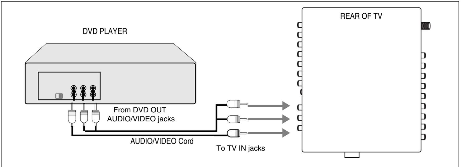
1. Connect the left and right audio cable from the DVD's Audio OUT jacks to the TV's audio left and right AV IN jacks. Connect the DVD's video OUT jack to the TV's video AV IN jack.
