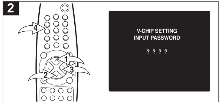
Press the CHANNEL UP ❶ or DOWN ❷ button until V-CHIP is selected, then press the VOLUME UP button ❸ to select it. Using the Direct Channel Selection buttons (0-9) ❹, enter the password ("0000" is the preset password if you have not changed it). This password can be changed to consist of different numbers (i.e. 1467, 3732) after the original password is entered.
