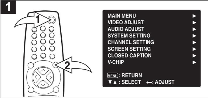
Press the POWER button ❶ to turn on the TV; the POWER indicator will light green. Press the MENU button ❷; the MENU screen will appear.
