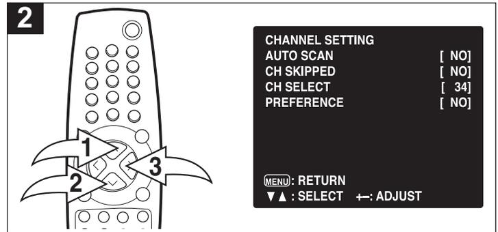
Press the CHANNEL UP ❶ or DOWN ❷ button until CHANNEL SETTING is selected, then press the VOLUME UP button ❸ to select it.
