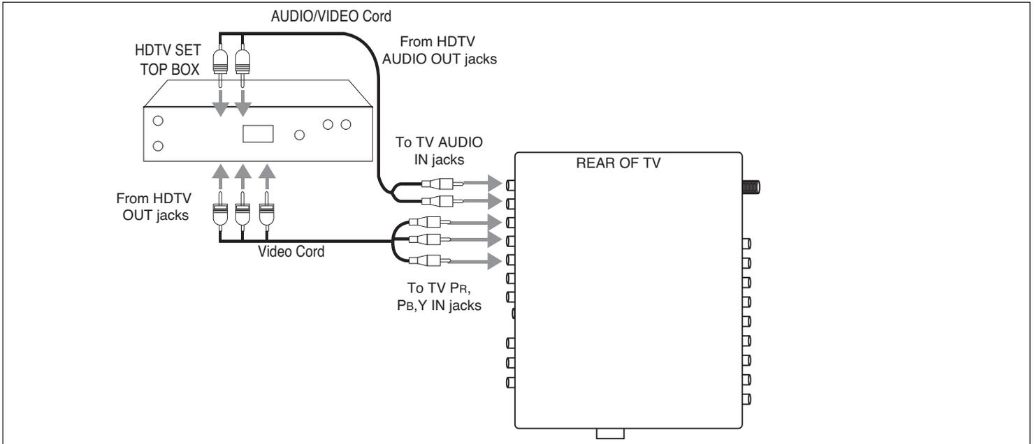
1. Connect the left and right audio cable from the HDTV's Audio OUT jacks to the TV's HDTV left and right Audio IN jacks.
