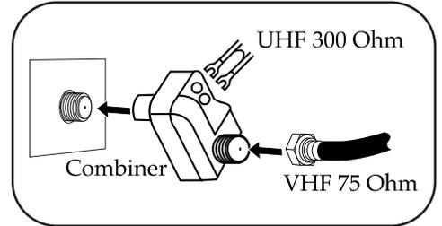
Connect the 75 ohm cable from the VHF antenna and the UHF antenna twin-lead wire to a combiner (NOT SUPPLIED). Attach the combiner to the antenna jack.
