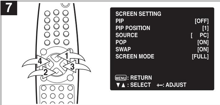
Press the CHANNEL UP **1** or DOWN **2** button until SWAP is selected. Turn this option ON or OFF using the VOLUME UP **3** or DOWN **4** button. If set to ON, the PIP/POP screens will swap.
