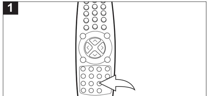
Press the SWAP button to alternate the screens when using PIP or POP. This will also alternate what screen the VOLUME, VIDEO SOURCE, etc buttons control.
