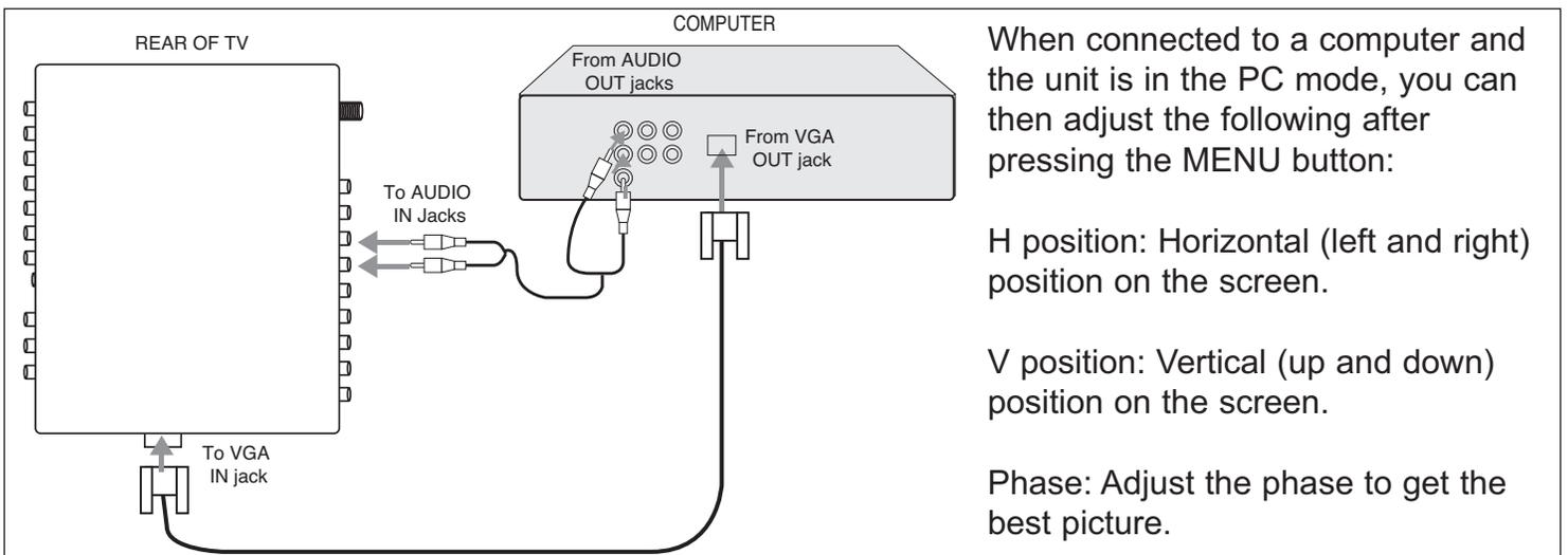
When connected to a computer and the unit is in the PC mode, you can then adjust the following after pressing the MENU button:
