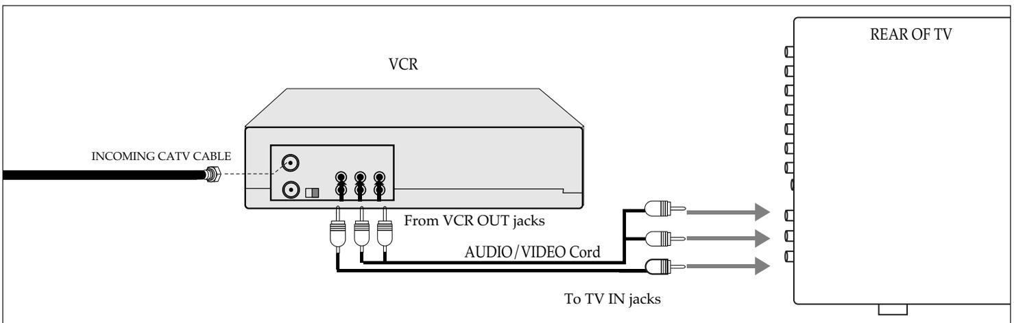
1. Connect the cable, satellite or incoming antenna to the VHF/UHF IN jack on the rear of the VCR.
