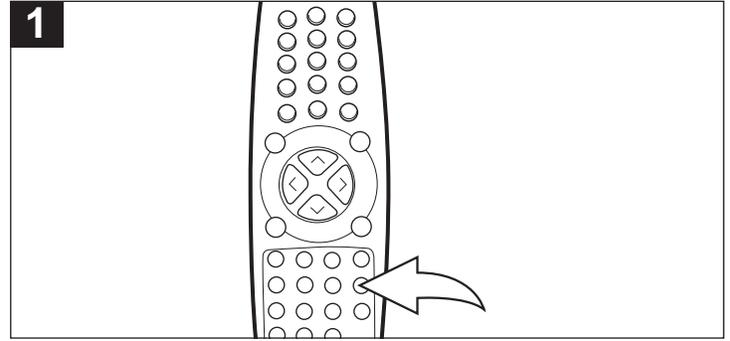
Each broadcasting channel has its own signal conditions and it is inconvenient to adjust the volume every time the channel is changed or when a commercial comes on. Audio AI automatically adjusts the volume of the desired channel by lowering the sound output when the modulation signal is high or by raising the sound output when the modulation signal is low. Press the AUDIO AI button to turn this feature on or off.
