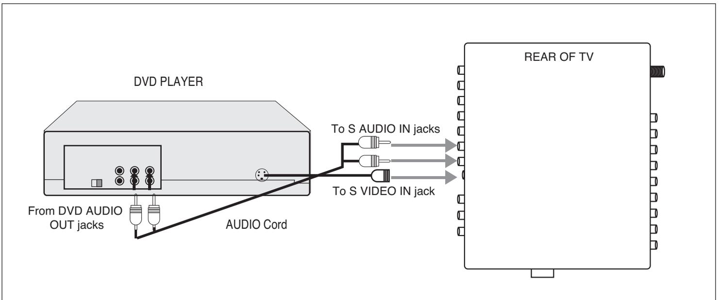
1. Connect the left and right audio cable from the DVD's Audio OUT jacks to the TV's audio left and right S IN jacks.
