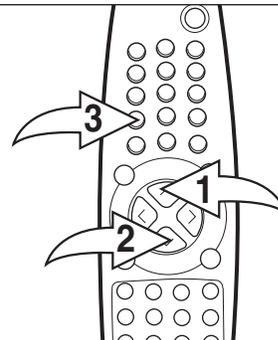
**For proper operation, before selecting channels, they must be set into the TV's program memory, see page 19.** Press and release the CHANNEL UP ❶ or DOWN ❷ button. The TV automatically stops at the next channel set into memory. This will not operate if channels are not set into memory.
