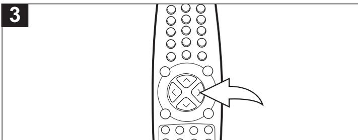
When AUTO MEMORY is selected, press the VOLUME UP button to start the Auto Search. The TV will automatically cycle through all the channels and store active channels into memory. When completed, the TV will be on the first available channel.
