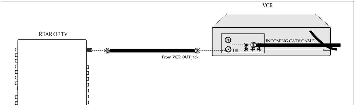
1. Connect the cable, satellite or incoming antenna to the VHF/UHF IN jack on the rear of the VCR.
