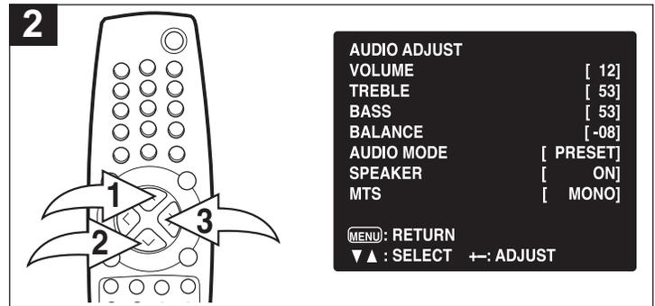
Press the CHANNEL UP ① or DOWN ② button until AUDIO ADJUST is selected, then press the VOLUME UP button ③ to select it. Press the CHANNEL UP ① or DOWN ② button until AUDIO MODE is selected.
