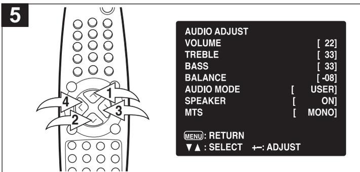
Press the CHANNEL UP ① or DOWN ② button until MTS is selected. Using the VOLUME UP ③ or DOWN ④ button, select the MTS setting (MONO or STEREO).
