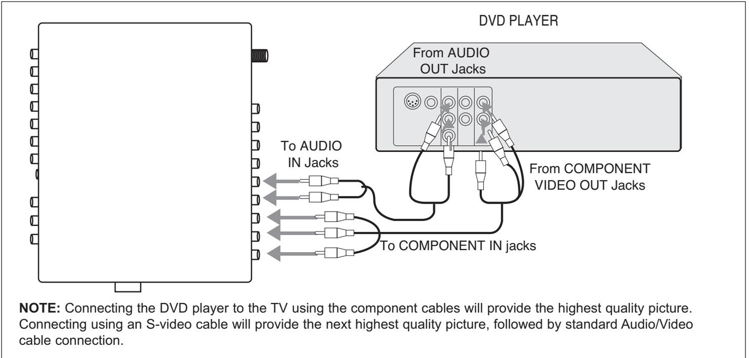
1. Connect the left and right audio cable from the DVD's Audio OUT jacks to the TV's audio left and right AV IN jacks.
