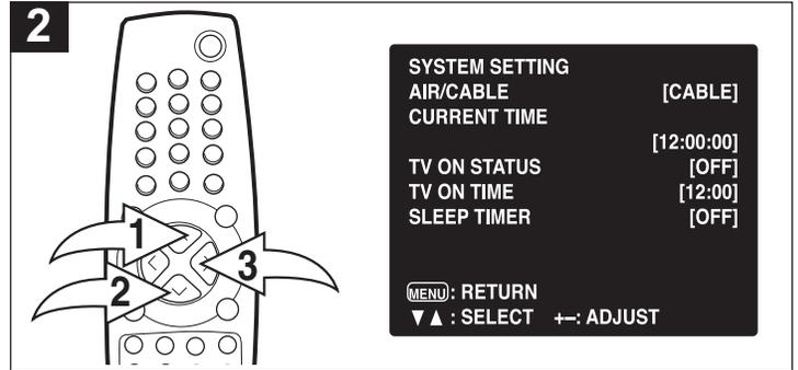
Press the CHANNEL UP ❶ or DOWN ❷ button until SYSTEM SETTING is selected, then press the VOLUME UP button ❸ to select it. Press the CHANNEL UP ❶ or DOWN ❷ button until CURRENT TIME is selected.
