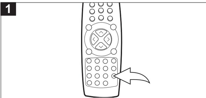
Press this button to select one of the four corners of the screen for the PIP picture.
