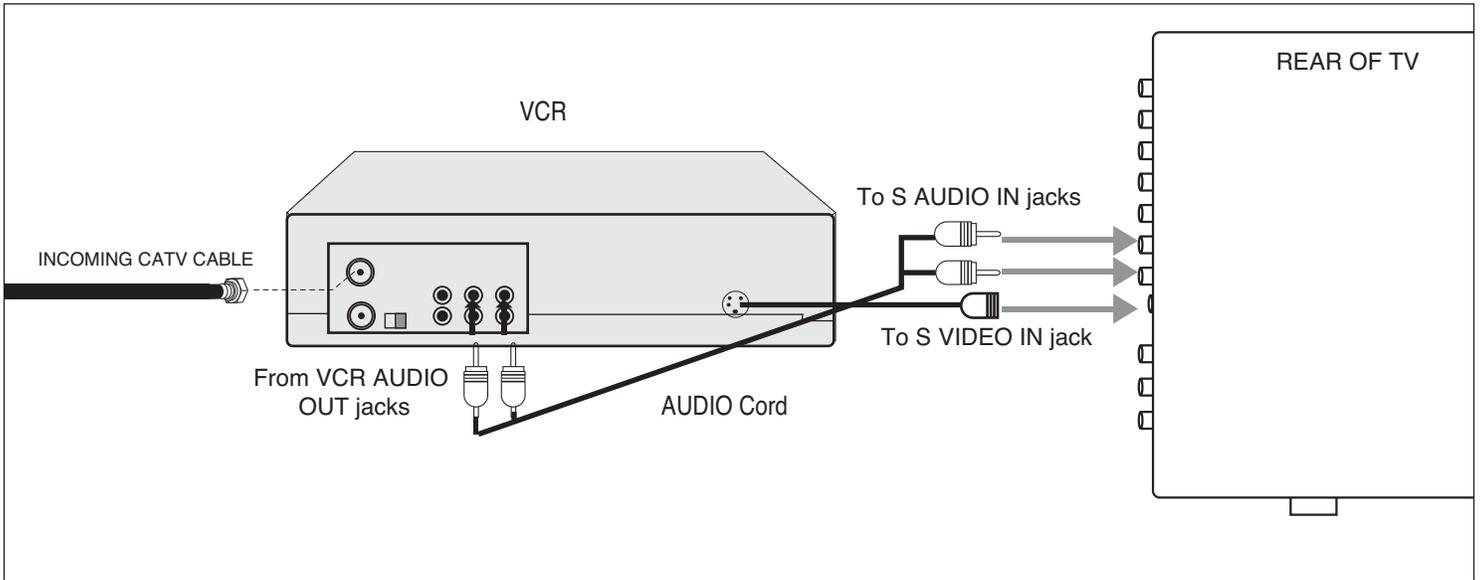
1. Connect the cable, satellite or incoming antenna to the ANT jack on the rear of the VCR.
