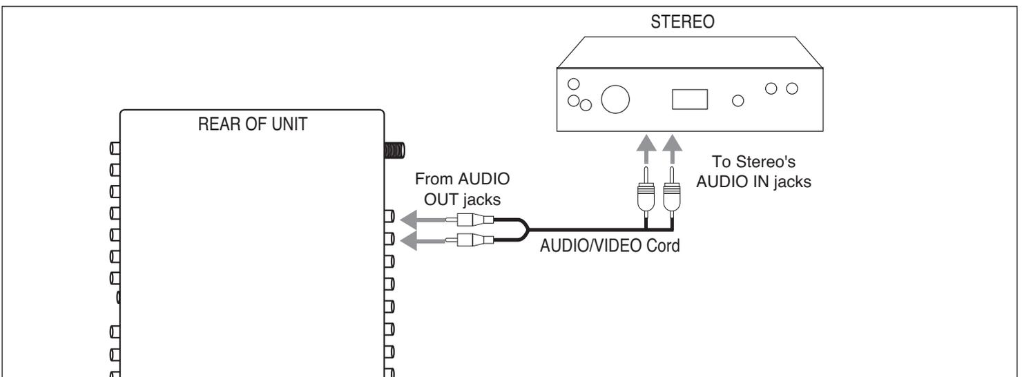
1. Connect the left and right audio cable from the TV's left and right Audio OUT jacks to the stereo system's left and right Audio IN jacks.
