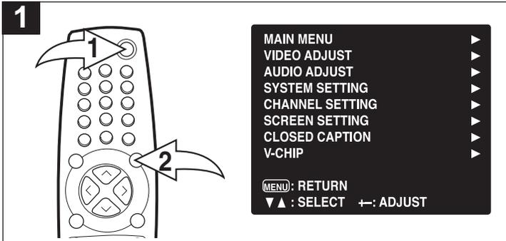
Press the POWER button **1** to turn on the TV; the POWER indicator will light green. Press the MENU button **2**; the MENU screen will appear.
