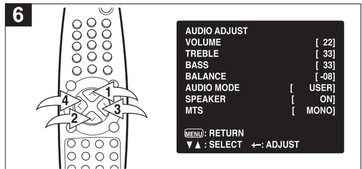
Press the CHANNEL UP ① or DOWN ② button until SPEAKER is selected. Using the VOLUME UP ③ or DOWN ④ button, turn this setting ON or OFF. Turn off if you want to use the external AUDIO OUT jacks on the rear of the set and mute the TV's built-in speakers.
