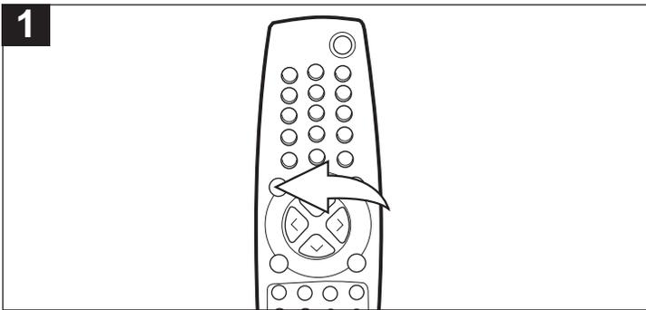
Repeatedly press this button to cycle through the device(s) connected to the INPUT jacks (TV/CATV, AV, S-VIDEO, COMPONENT, YPbPr and PC).
