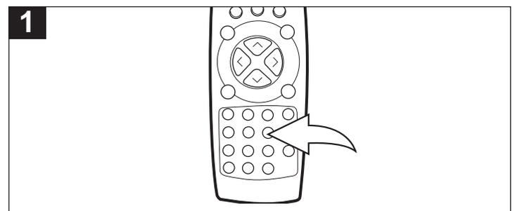
Press repeatedly to set the sleep time between "00" and "90" (each press will increase the time by 10 minutes). When the sleep time is up, the TV will shut off. Select "00" to cancel the sleep function.
