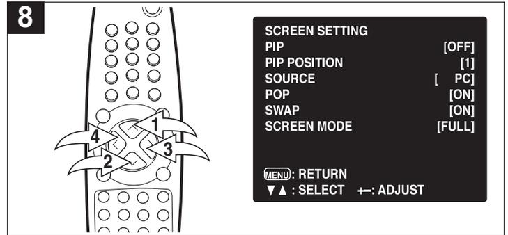
Press the CHANNEL UP **1** or DOWN **2** button until SCREEN MODE is selected. Press the VOLUME UP **3** or DOWN **4** button to select one of the screen modes as follows:
