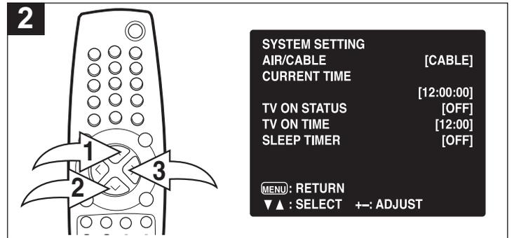
Press the CHANNEL UP ❶ or DOWN ❷ button until SYSTEM SETTING is selected, then press the VOLUME UP button ❸ to select it. Press the CHANNEL UP ❶ or DOWN ❷ button until AIR/CABLE is selected.
