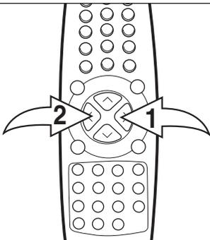
Adjust the volume level by pressing the VOLUME UP ❶ or DOWN ❷ button. The volume level will be indicated on the screen by a green numerical display between 0 and 100 where 0 is the lowest setting and 100 is the loudest.
