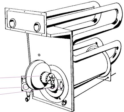
**Drum and Tube Heat Exchanger**
