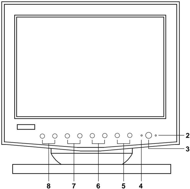
1. **Master Power** (On rear): Push to provide power to the monitor. This switch should be left ON for daily operation. Use the front panel On/Off control **(3)** to turn the monitor display on and off.
