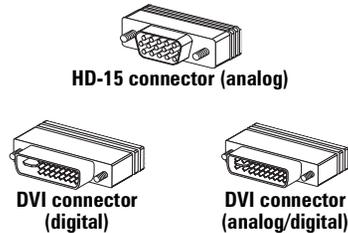
Some monitors with DVI connectors support both digital and analog input. If you're using one of these monitors with your Matrox product, make sure it's configured to use the correct type of input. For more information, see your monitor documentation.
