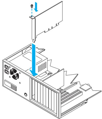
Your Matrox card is now installed. *Before restarting your computer*, connect your monitor or monitors (see “[Connection setup](#)”, page 4). *After connecting*, restart your computer and install your Matrox software (see “[Software installation](#)”, page 8).
