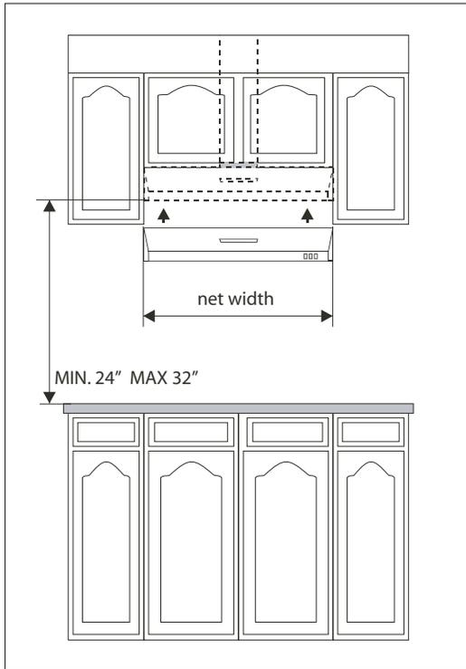
Minimum mount height between range top to hood bottom should be no less than 24".
