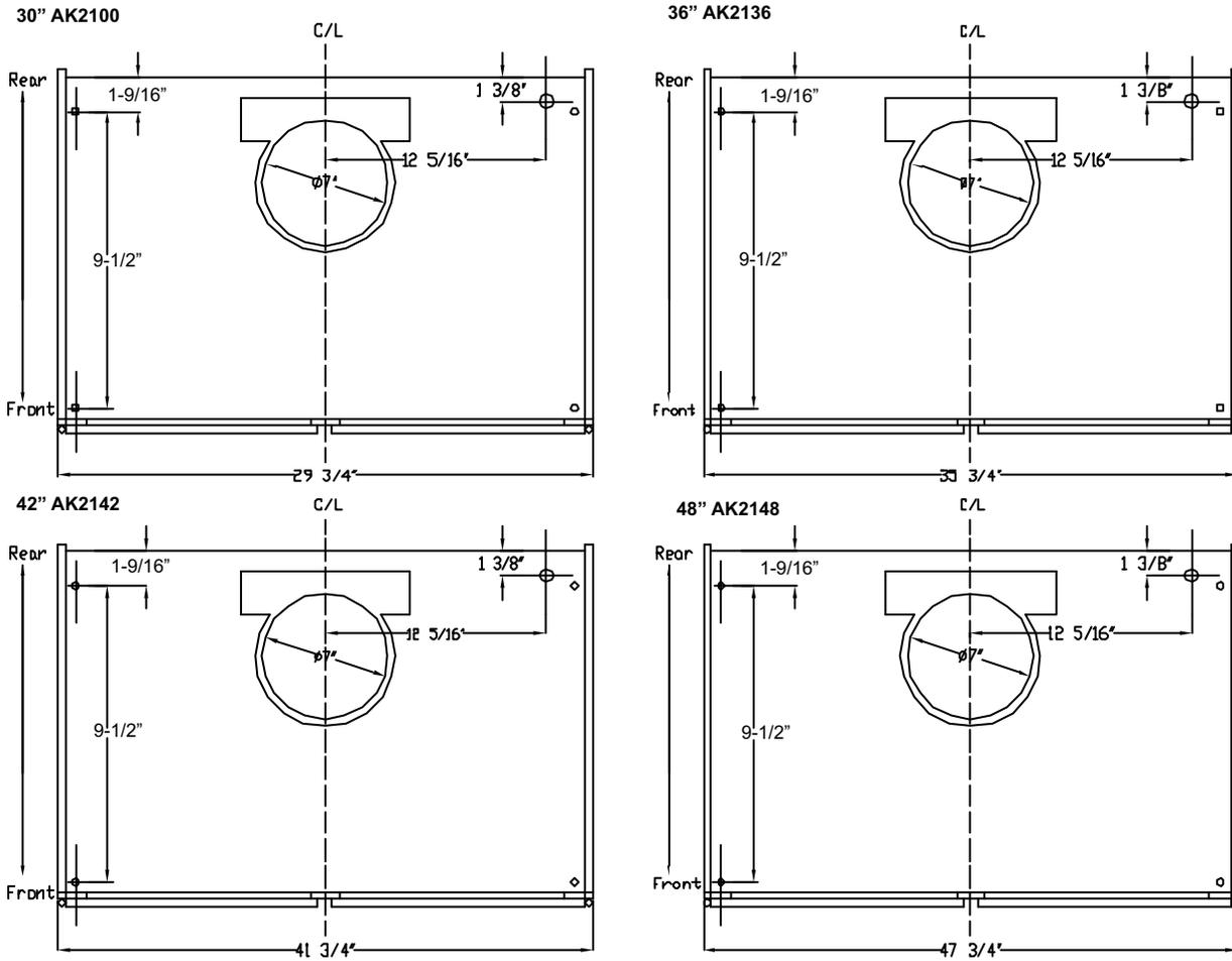
\* Dimensions for electrical knockout and mounting holes are the same for all units.
