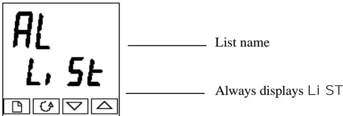
Figure 2-5 Typical list header display
