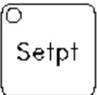
This key selects the Setpoint Enter mode where the Setpoint, Setpoint Offset and Reference Number can be accessed and altered. When used in the dual-key operation Shift/Setpt it allows the operator to pull any program into the edit space or decrease the remaining time of a program step if a program is currently running.
