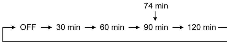
Note: When the sleep timer has only 1 minute left, an OSD “SLEEP 1 min.” will automatically appear and stay on the screen. When the sleep timer counts down to 0, the receiver automatically shuts down by itself to standby mode.
