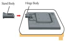
3. Assemble the Stand Base(Front, Rear) into the Stand Body in the correct direction.
