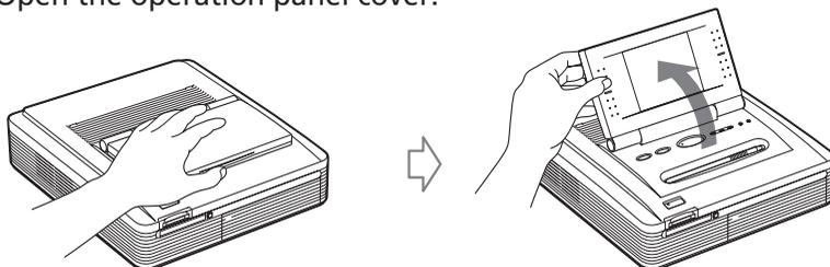
You can rotate the operation panel up to 180 degrees. Use the panel at an appropriate angle such that you can view the screen clearly and can perform the stylus operations easily.
