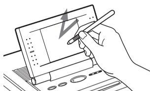
Move the stylus while pressing on an image or item on the operation panel screen using the point of the supplied stylus.
