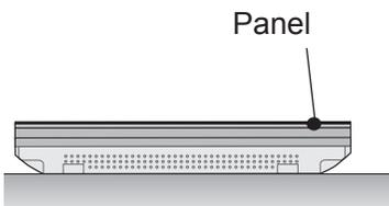
If there is not a cushion available, ensure the floor is clean and then lay the product down carefully with the panel facing either upward or downward. At this time, be careful for objects not to fall on the panel.
