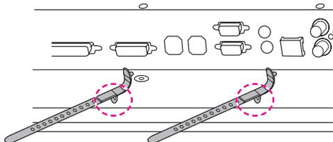
As illustrated, screw the power cable holder into the hole on the bottom rear of the set to hold the power cables together. (This is to put the power cables inside the holder.)
