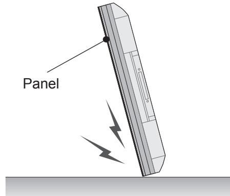
If the product is tilted onto the bezel, the bottom of the panel may be damaged.
