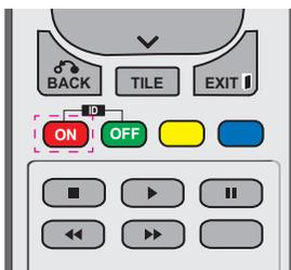
2 If you press the left/right buttons or press the ON button repeatedly, the Picture ID cycles through OFF and 1 to 4. Assign the ID you want.
