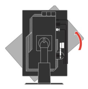
Place the cables through the Main Clip. Then fasten the clip.
